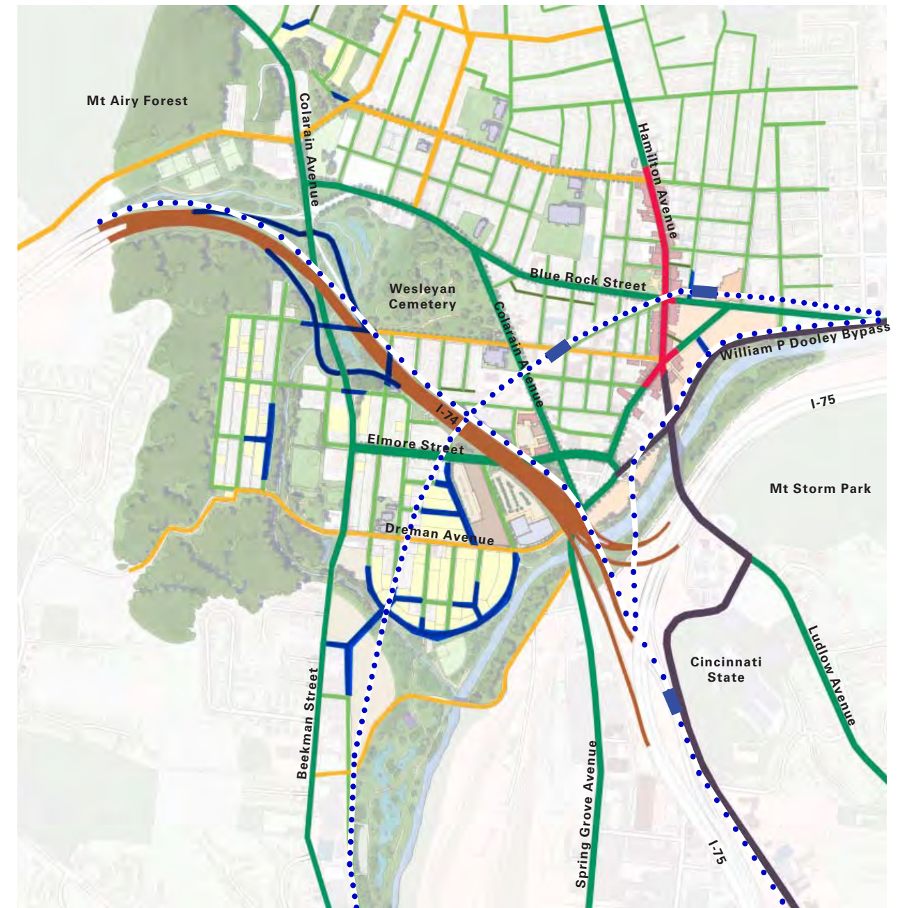
STREET CLASSIFICATIONS This diagram depicts the proposed street hierarchy and potential transit alignments. See page 76 of Transportation and Infrastructure Appendix for detailed descriptions. ■ GREAT STREET ■ NEW INTERCHANGE ■ OTHER SIGNATURE STREET ■ MAIN STREET ●●●● OPTIONAL TRANSIT ALIGNMENTS ■ NEIGHBORHOOD STREET ■ RESIDENTIAL STREET
