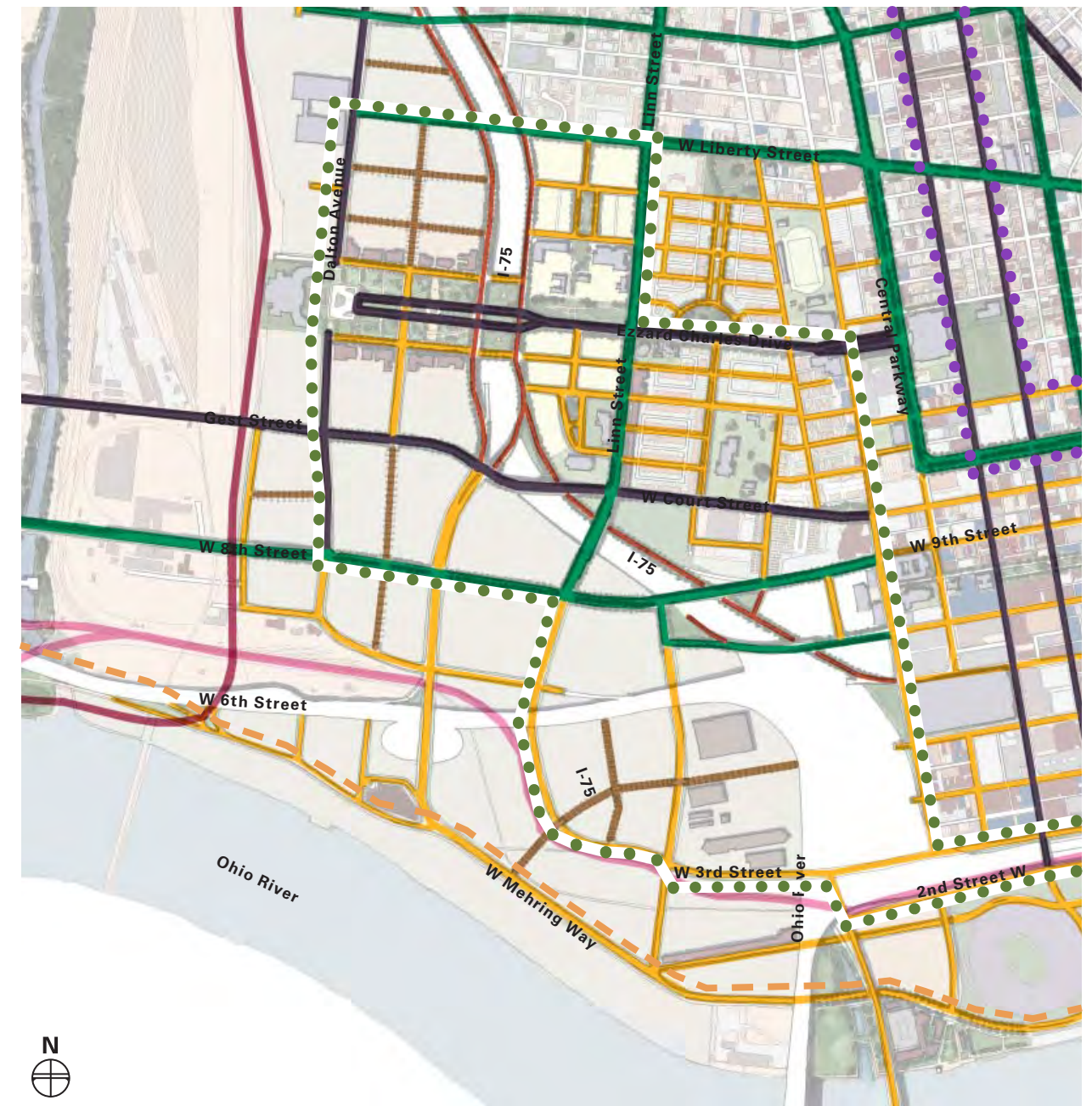
TRANSPORTATION NETWORK This diagram depicts the various road types and proposed passenger and light rail alignment for the proposed plan. See page 76 of Transportation and Infrastructure Appendix for detailed descriptions. ■ LOCAL COLLECTOR STREET ■ OTHER SIGNATURE STREET ■ TRANSIT ■ GREAT STREET ■ NEIGHBORHOOD STREET ■ PASSENGER RAIL ■ OPTIONAL STREET ■ BICYCLE TRAIL ●●● QUEENSGATE STREET CAR ●●● DOWNTOWN STREET CAR
