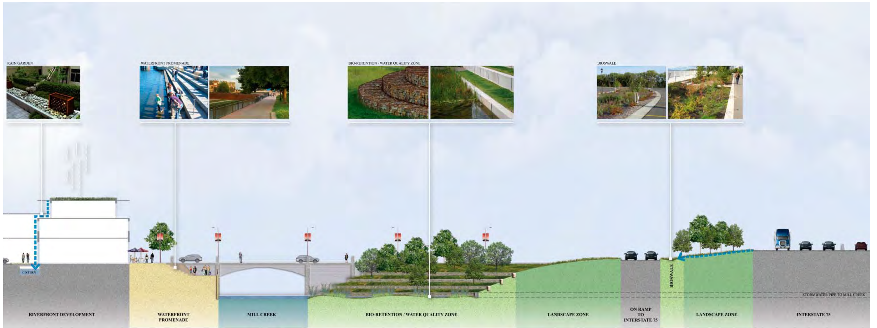
MITCHELL AVENUE SECTION The section illustrates how the Mill Creek could be slightly modified to increase sustainable practices for water quality and conveyance in a way that provides amenity for future development but scenic beauty for the many travelers who use the I-75 corridor.
